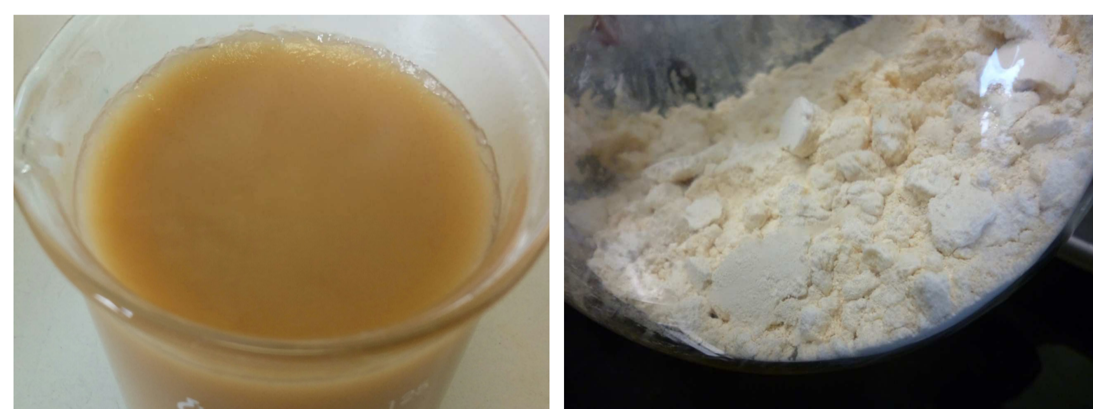
Figure 3: Separated PA6 matrix. Polymer solution (left) and dried polymer after solvent recovery (right)
