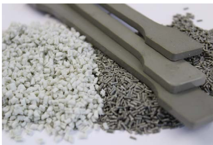
Figure 7. Recovered PBT material from CreaSolv ® Process after solvent recovery: PBT-blend (left) and pure recyclate (right).
