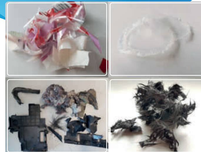
Waste to new materials – treatment of end of life flexible film and automotive scrap yield both high purity mono-polymers and recovered reinforcing fibres
