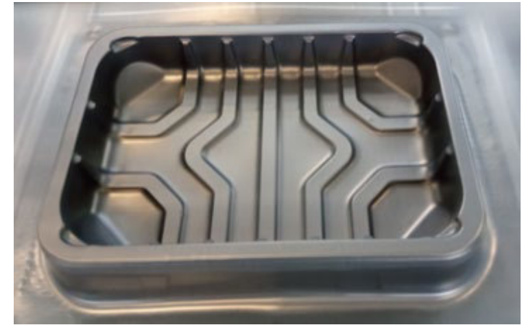
Figure 2.2 Demonstrator from NONTOX from small scale Thermoforming validation trials (TRL4)
