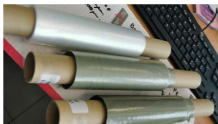
Monolayer blown film rolls with (top to bottom) 100% virgin, 50% r-PE and 100% r-PE content
